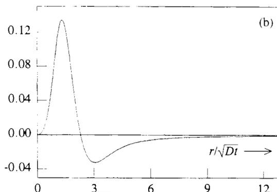
Fig. 5. The product of the normalised current density difference ( $i_{cyl} - i_{model}$ ) plotted versus  $r/\sqrt{Dt}$  for semi-apical angles (a)  $\theta_0 = 3\pi/4$  and (b)  $\theta_0 = \pi/4$ . The integration of these functions, see Eq. (47), generated two of the points in Fig. 1.
