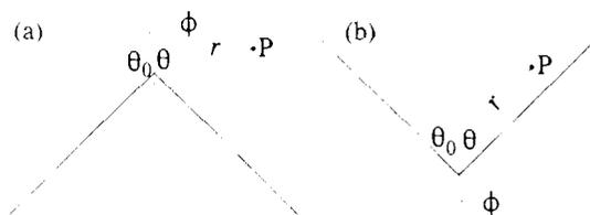
Fig. 1 The coordinate system used to designate the position of P, an arbitrary point in solution. In (a) a spired electrode penetrates into the surrounding solution:  $\pi/2 < \theta_0 < \pi$ . In (b) the solution occupies the depression in a cavernous electrode:  $0 < \theta_0 < \pi/2$ .
