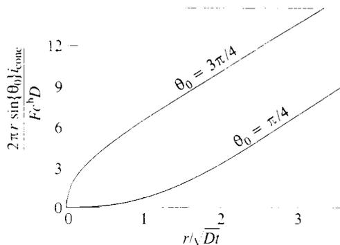
Fig. 2. The product of current density and perimeter length, normalised by division by  $Fc^b D$ , at a distance  $r$  from the apex of a cone, plotted as a function of  $r/\sqrt{Dt}$  for the semi-apical angles  $\theta_0 = 3\pi/4$  and  $\pi/4$ .
