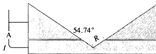
Fig. 3. Diagram of a device that will give a long-time current response independent of the diffusivity of the electroactive species but proportional to its concentration.
