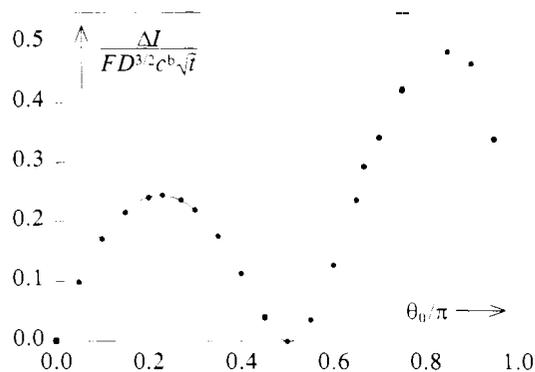
Fig. 1. Graph, versus the semi-apical angle  $\theta_0$ , of the difference between the current at an infinite cone and that at the cylindrical model of an infinite cone. The current difference increases with time and has been normalised by division by  $FD^{3/2}c^b/\sqrt{t}$ .
